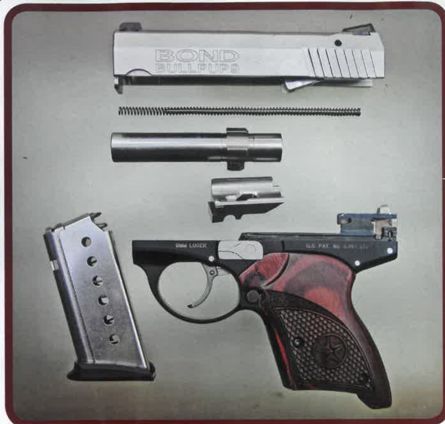
The Bullpup9, fieldstripped. The part below the barrel is the rotation base. It's best to refer to the owner's manual during your first attempts at disassembly.
